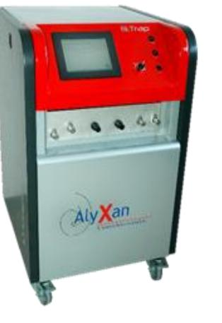
compact FTICR mass We have developed spectrometers ; first in the LCP lab, now commercialized by AlyXan. Our instruments use permanent magnets in order to generate the magnetic field (nominal field up to 1.5 Tesla).
