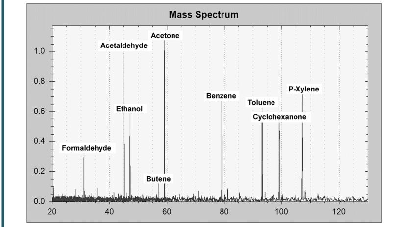
When using chemical ionization (here proton transfer from  $H_30^+$  ions) one peak is observed for each species present.
