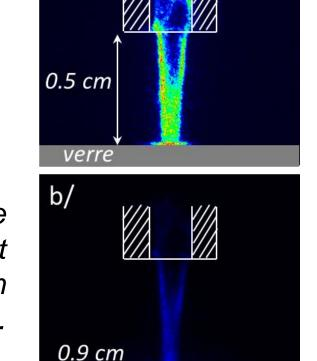
Effect of the presence of a glass surface placed 5mm away from the capillary exit At longer times the plasma spreads on the surface.
