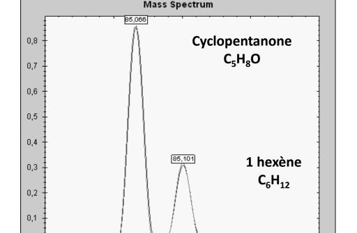
The high resolution allows a precise identification of the organic molecules that are present, even when they are at very low concentrations.
