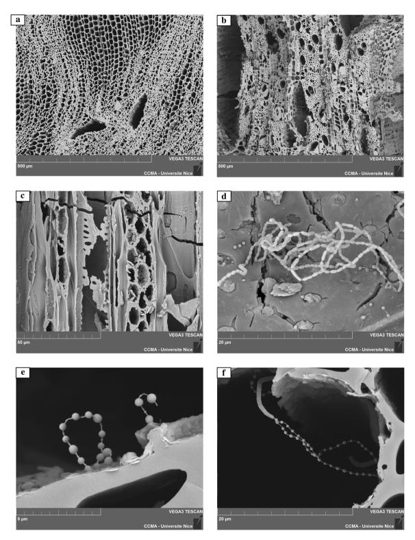
Figure 6: Scanning electron micrographs. (a) Pinus type sylvestris, cross-section: example of FA. (b) Prunus type 2, crosssection: example of RC. (c) Prunus type 1., tangential section: example of FA. (d, e, f) Examples of micro-organisms: tangential section of Acer (d), cross-section (e) and tangential section (f) of  $\emph{Viburnum}$ .
