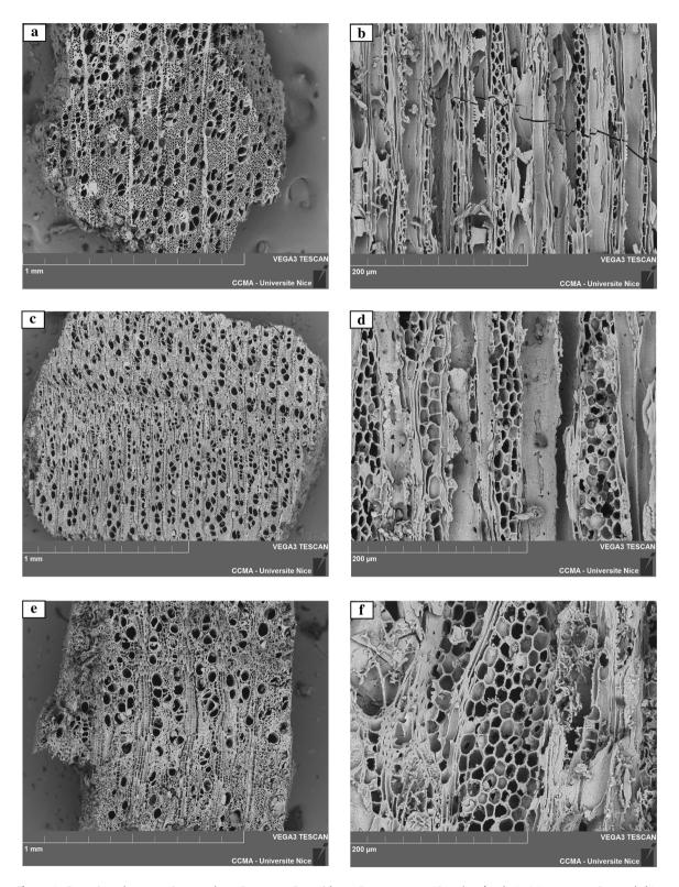
Figure 4: Scanning electron micrographs – Rosaceae Prunoideae. Prunus type 1 (P. avium/padus): (a) cross-section and (b) tangential section. Prunus type 2 (P. mahaleb/padus/spinosa): (c) cross-section and (d) tangential section. Prunus type 3 (P. amygdalus/spinosa): (e) cross-section and (f) tangential section.
