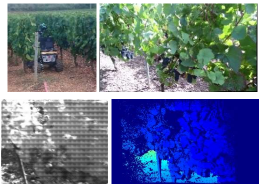
Fig. 1. Top-left: Summit XL mobile robot instrumented with the multi-sensors system; Top-right: RGB image; Bottom left: MS image; Bottom right: Depth image.
