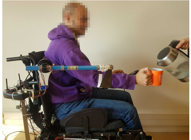
Fig. 1: The active DAS prototype used to implement the four proposed strategies to compensate for the upper-limb weight.
