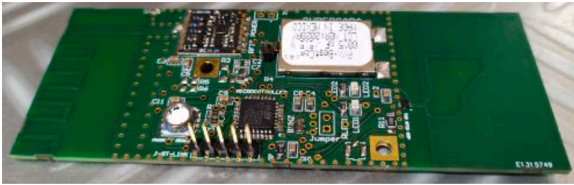
Fig. 5. Smart-tag prototype (respectively IFA on the left and slot antenna on the right).
