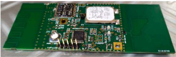
Fig. 5. Smart-tag prototype (respectively IFA on the left and slot antenna on the right).
