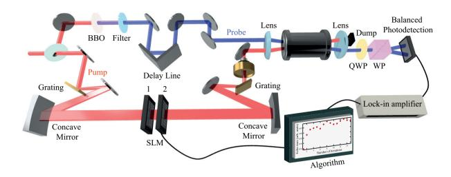
**Figure 1** Experimental pump-probe setup used to create a bipulse and optimize the echo amplitude. SLM: one-dimensional dual mask liquid crystal spatial light modulator, P: Glan polarizer, QWP: quarter waveplate, WP: Wollaston prism.
