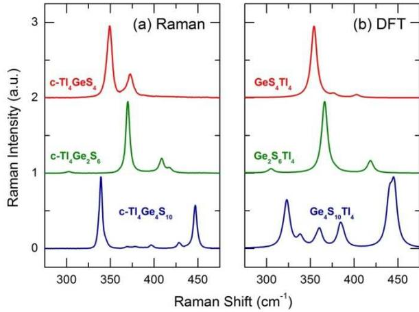
Figure 2. (a) Experimental Raman spectra of the crystalline reference compounds Tl<sub>4</sub>Ge<sub>4</sub>S<sub>10</sub> ( $x = \frac{1}{3}$ ), Tl<sub>4</sub>Ge<sub>2</sub>S<sub>6</sub> ( $x = \frac{1}{2}$ ), and Tl<sub>4</sub>GeS<sub>4</sub> ( $x = \frac{2}{3}$ ) within the Ge-S stretching spectral domain, and (b) DFT Raman spectra of the respective Tl-Ge-S clusters.
