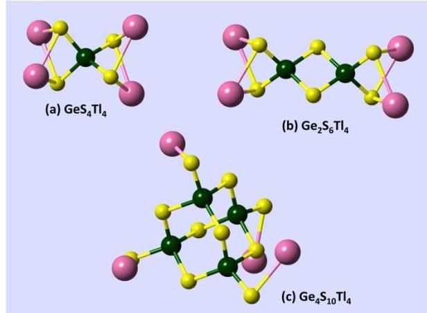
Figure 3. Optimized geometry of the Tl-Ge-S clusters: (a) GeS<sub>4</sub>Tl<sub>4</sub>, (b) Ge<sub>2</sub>S<sub>6</sub>Tl<sub>4</sub>, and (c) Ge<sub>4</sub>S<sub>10</sub>Tl<sub>4</sub>, used for DFT modelling of vibrational spectra of the crystalline reference compounds Tl<sub>4</sub>GeS<sub>4</sub>, Tl<sub>4</sub>Ge<sub>2</sub>S<sub>6</sub>, and Tl<sub>4</sub>Ge<sub>4</sub>S<sub>10</sub>, respectively.
