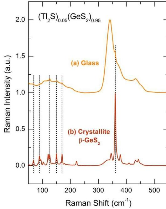
Figure 5. Raman spectra of (a)  $(\text{Tl}_2\text{S})_{0.05}(\text{GeS}_2)_{0.95}$  glass and (b) crystalline impurities of high-temperature  $\beta\text{-GeS}_2$ , found on the surface of the  $x = 0.05$  sample.
