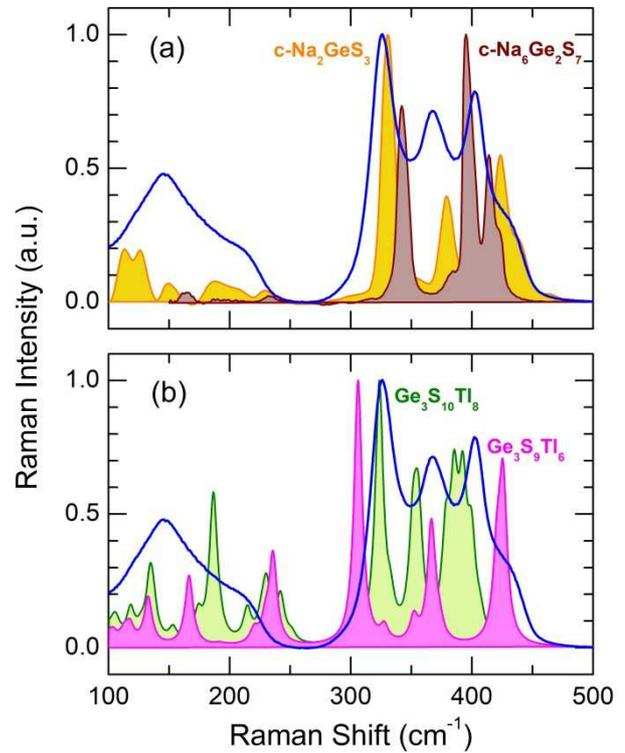
Figure 8. Experimental Raman spectra of the  $x = 0.5$  glass and (a) crystalline references c-Na<sub>2</sub>GeS<sub>3</sub> and c-Na<sub>6</sub>Ge<sub>2</sub>S<sub>7</sub> [34]; (b) DFT Raman spectra of Ge<sub>3</sub>S<sub>10</sub>Tl<sub>8</sub> and Ge<sub>3</sub>S<sub>9</sub>Tl<sub>6</sub> clusters.
