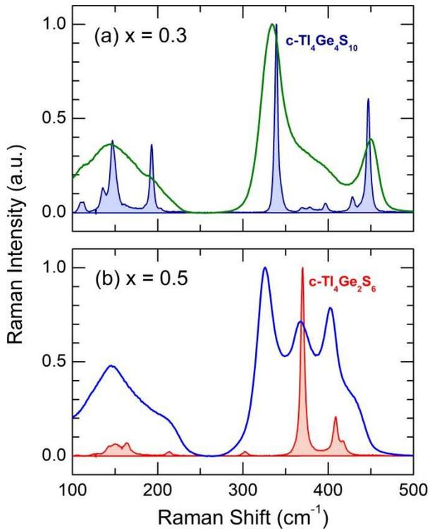
Figure 7. Experimental Raman spectra of (Tl<sub>2</sub>S) <sub>$x$</sub> (GeS<sub>2</sub>)<sub>1- $x$</sub>  glasses in comparison with respective crystalline compounds: (a)  $x = 0.3$  and c-Tl<sub>4</sub>Ge<sub>4</sub>S<sub>10</sub> ( $x = \frac{1}{3}$ ); (b)  $x = 0.5$  and c-Tl<sub>4</sub>Ge<sub>2</sub>S<sub>6</sub> ( $x = \frac{1}{2}$ ).
