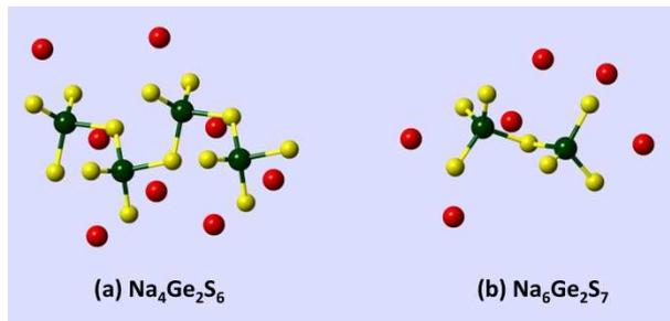
Figure 9. The crystal structure of (a) monoclinic  $\text{Na}_2\text{GeS}_3 = \text{Na}_4\text{Ge}_2\text{S}_6$ , space group  $P2_1/c$  [33], and (b) monoclinic  $\text{Na}_6\text{Ge}_2\text{S}_7$ , space group  $C2/c$  [46].
