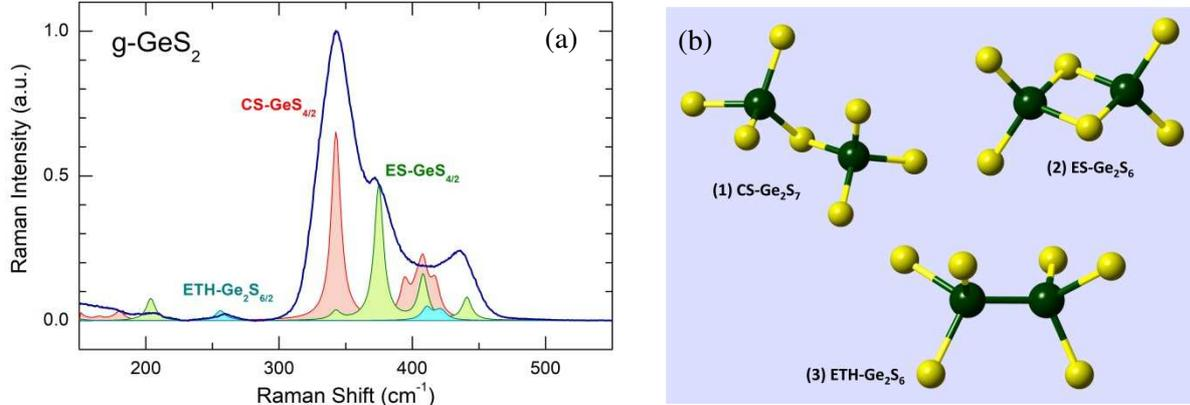
Figure 4. (a) Experimental Raman spectrum of glassy  $GeS_2$  and DFT Raman spectra of corner-sharing  $CS-GeS_{4/2}$  and edge-sharing  $ES-GeS_{4/2}$  tetrahedra, as well as of ethane-like  $ETH-Ge_2S_{6/2}$  units [35]; (b) schematic representation of (1)  $CS-Ge_2S_7$ , (2)  $ES-Ge_2S_6$ , and (3)  $ETH-Ge_2S_6$  clusters used for DFT modelling. The terminal hydrogen species are not shown and H-related vibrational modes are removed from the DFT spectra.
