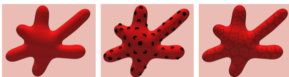
Figure 11: Organic-looking tessellation of surfaces. a) Shape to texture; b) User-selected kernels; c) Result.
