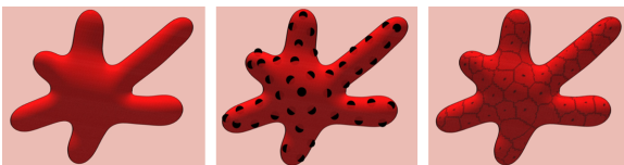
Figure 11: Organic-looking tessellation of surfaces. a) Shape to texture; b) User-selected kernels; c) Result.
