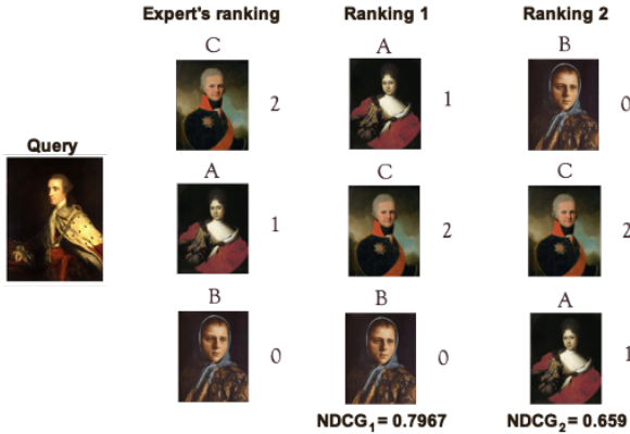
Figure 2. Calculated NDCG metrics for two rankings, expert’s ranking is the ranking with objects ranked in the most relevant order according to the expert’s criterion, 2, 1, 0 — the relevance scores rel_i in the ground truth ranking.
