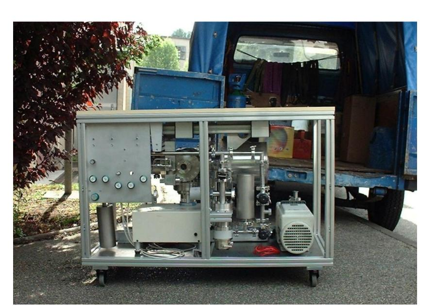
The InfraRed Multiphoton Dissociation experiments are realised with a Mobile Ion Cyclotron Resonance Analyzer (MICRA), associated to the Orsay Free Electron Laser CLIO. The mass spectrometer is based on the use of a permanent magnet assembly (Halbach cylinder) producing a nominal magnetic field of 1.25T.
