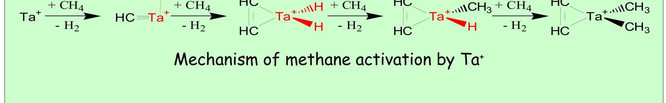
IRMPD has been used to characterize the mechanism of the sequential dehydrogenation of four methane molecules by third row transition metal cation Ta<sup>+</sup>.
