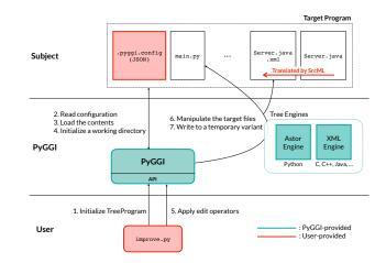
Figure 1: Workflow of PyGGI 2.0 for tree-based programs
