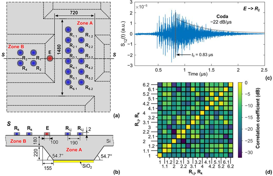
**FIG. 3.** (a) Scheme of a field confinement region and disposition of the ZnO transducers. (b) Side view S of the upper figure. (c) Impulse response  $S_{12}(t)$  between E and  $R_2$ . (d) The cross-correlation coefficients for the total of considered receivers.
