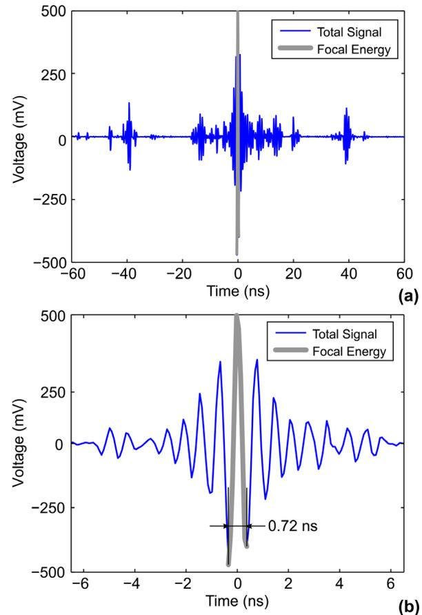
**FIG. 5.** Calculating the compression ratio for signal on  $R_2$  obtained using deconvolution. (a) Ratio of the energy in the main peak to the total energy. (b) Zoom of the central peak.
