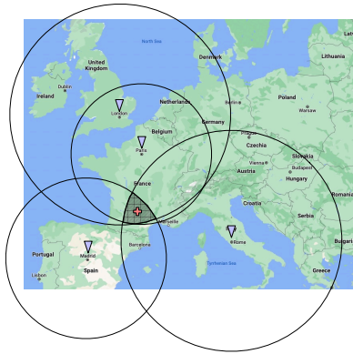
(a) Tier 1 performs CBG from VPs to the target, compute the centroid of the intersection that will serve for Tier 2.
