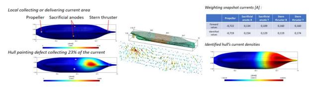
Figure 1: left column: Forward modelling of the hull (top: delivering localized current areas, down: paint defect current density). Middle column: noisy electric field computed signature. Right column: solution of the inverse problem (top: forward and identified snapshot weighting current, down: identified current hull's current density).
