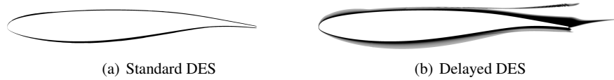
Fig. 2 Regions of RANS (in black) and LES (in white) modes around the OAT15A profile
