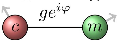
Figure 1: Representation of the magnon/photon coupling. Coupling phase  $\varphi$  measures the difference in direction of the (local) yellow arrows.
