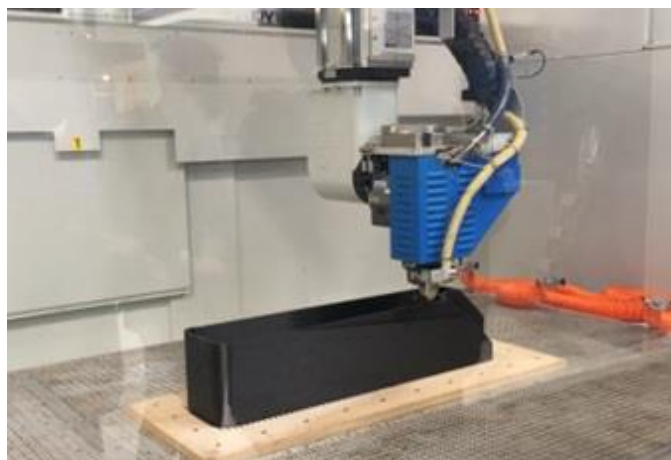
Fig. 9 3D printing of carbon-composite compound (court. of CMS)
