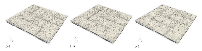
Figure 9: Orientation distribution of the material frame of the tows in the woven microstructure: (a)  $e_1$ ; (b)  $e_2$ ; (c)  $e_3$ .
