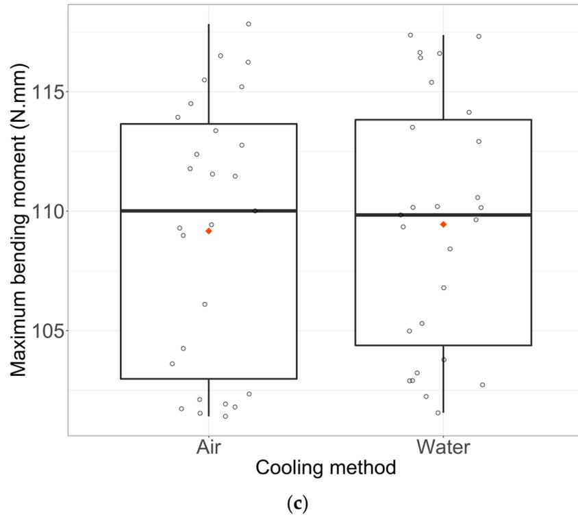
**Figure 5.** Boxplots of Y1 (Maximum bending moment) with the simple effect of factors u1 (a), u2 (b), and u3 (c). Each boxplot plotted in black shows the median and quartiles (rectangle widths stand for 25% and 75% quartiles) and points in dark stand for extreme values. Data points are shown and the mean is represented by a red lozenge.
