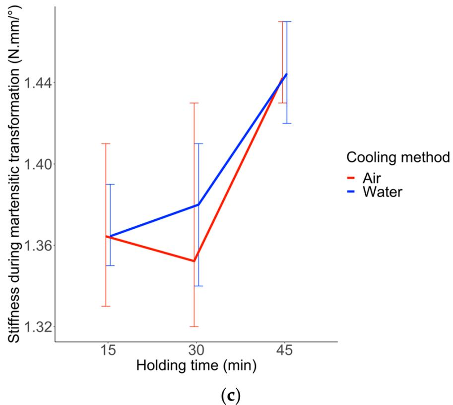
**Figure 10.** Interaction plot for each pair of factors for response Y3. (a) interaction u1 and u2 (temperature and holding time). (b) interaction u1 and u3 (temperature and cooling method). (c) interaction u2 and u3 (holding time and cooling method). The extremities of the associated vertical line stand for 25% and 75% quartiles.
