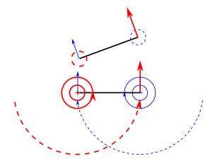
**Figure 4.** Interaction of two unequal monopolar vortices of opposite signs. A stronger positive vorticity vortex on the left, results in a counter-clockwise rotation as it drags the weaker vortex along its streamlines. If the weaker vortex was very small it would be advected by the flow of the larger vortex like a passive scalar. Note that the initial part of the cartoon also works for understanding the effect of a sheared flow on the dipole vortex.
