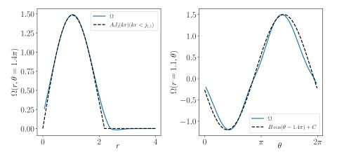
**Figure 9.** The radial and the poloidal profiles of the dipole vortex of Figure 8. The solid lines show the numerical forms, whereas the dashed lines are the analytical expressions. The dashed line on the left is  $\Omega(r) = AJ_1(kr)$ , with A = 2.55 and k = 1.75, up to the first zero of  $J_1(kr)$  (i.e.  $kr < j_{1,1}$ ) and zero afterwards, whereas the one on the right is  $\Omega(\theta) = C \cos(\theta - 1.4\pi) + D$ , with C = 1.35 and D = 0.15.
