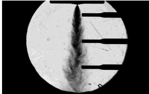
Figure 9. Visualization of the thermocouple location.
