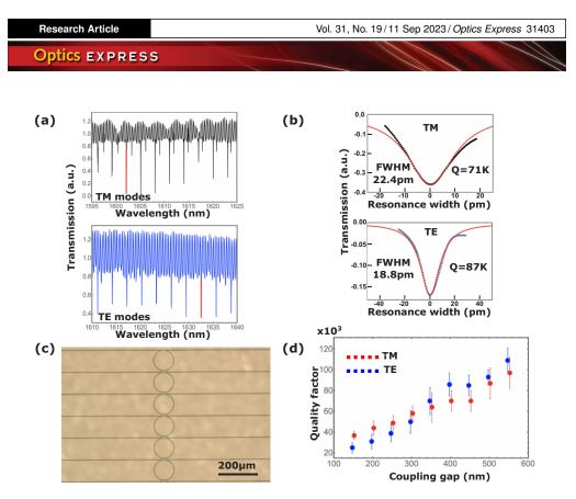
**Fig. 4.** (a) Typical transmission spectra of a ring resonator for TM and TE modes. (b) Zoom on narrow resonances corresponding to the TM and TE modes in the ring with Lorentzian fit of the data given by the red curves. (c) Microscope image of a group of ring resonators with varying coupling gaps. (d) Loaded quality factors of the ring resonators as a function of the coupling gap between a ring and a waveguide.
