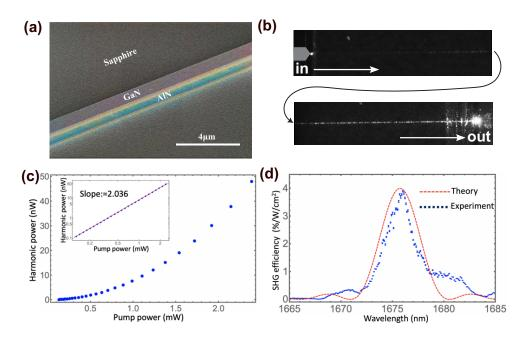
**Fig. 5.** (a) SEM image of the waveguide used for the SHG experiment. (b) Images of the second harmonic generation in the 4.5 mm long waveguide. Since the waveguide is long, only entrance (top) and exit (bottom) parts are shown. (c) Power of the second harmonic as a function of the injected pump power. Linear fit of the log plot shows a quadratic dependence corresponding to the second harmonic generation. (d) Normalized second harmonic efficiency as the function of the pump wavelength.
