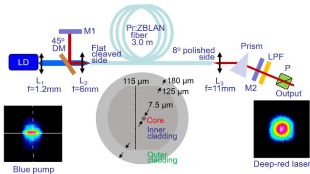
**Fig. 4.** Scheme of the diode-pumped double-clad deep-red fiber laser: M1 – rear mirror, M2 – output coupler, LD – laser diode, L<sub>1-3</sub> – lenses, DM – dichroic mirror (45°), LPF – long-pass filter, P – polarizer, *inset* – cross-section of the double-clad fiber. *Insets* – beam profiles of the pump (at the input fiber facet) and laser radiation (in the far-field).
