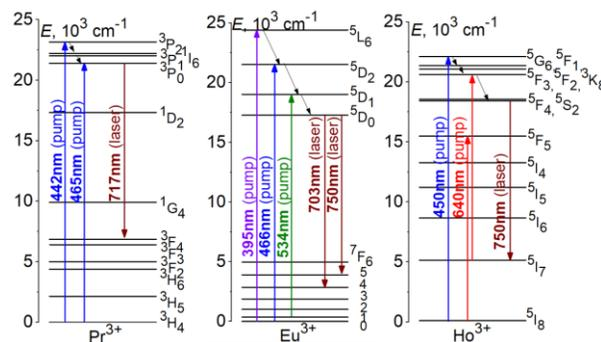
**Fig. 1.** Energy-level schemes of Pr<sup>3+</sup>, Eu<sup>3+</sup> and Ho<sup>3+</sup> ions showing pump and deep-red laser transitions.
