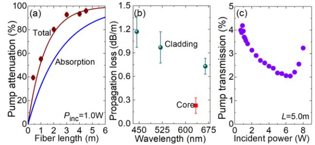
**Fig. 3.** Characterization of the double-clad Pr<sup>3+</sup>-doped fluoride fiber: attenuation of the pump radiation from a GaN diode vs. the fiber length at  $P_{\text{inc}} = 1.0$  W: symbols – experimental data, curves – simulation: pump absorption and losses (solid curve), pump absorption only (dashed curve); (b) propagation losses for the fiber inner cladding and core; (c) pump transmission vs. the incident pump power for a 5.0 m-long fiber.
