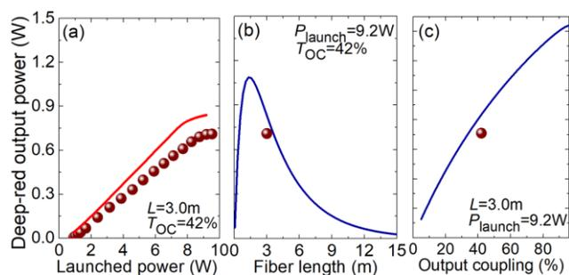
**Fig. 7.** Simulated output power of a deep-red Pr fiber laser: (a) vs. the launched pump power,  $L = 3.0$  m,  $T_{OC} = 42\%$ ; (b) vs. the fiber length,  $T_{OC} = 42\%$ ,  $P_{\text{launch}} = 9.2$  W; (c) vs. the output coupling,  $L = 3.0$  m,  $P_{\text{launch}} = 9.2$  W, circles – experiment, curves – simulation. Other simulation parameters are listed in the text.
