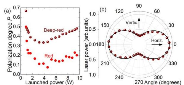
**Fig. 6.** Polarization effects in the deep-red / red double-clad Pr fiber lasers: (a) polarization degree ( $P$ ) of laser emission; (b) normalized polar plot of the polarization-dependent output power for the deep-red laser, **launched pump power:**  $P_{launch} = 9.2$  W.
