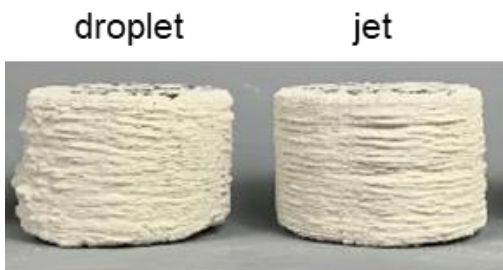
248 Figure 14: Comparison of printed cylinders (diameter: 60mm, height: 40mm) with droplet and liquid jet application
