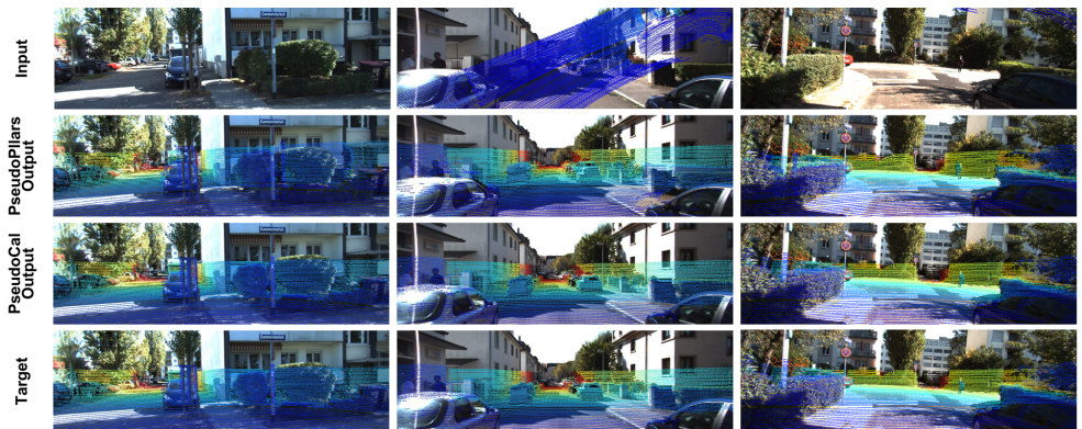
Figure 6: Qualitative evaluation of PseudoCal on KITTI (best viewed on screen). The point clouds are color-coded according to depth. Rows represent the initial decalibrations, PseudoPillars’ coarse adjustments, PseudoCal’s final refined calibrations, and groundtruth.
