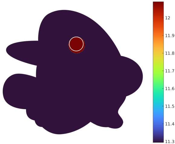
Figure 7: Real part of the reconstructed refractive index in the geometry of a 2D head profile in microwave regime. The boundary of the exact support of the perturbation is shown as a white line.
