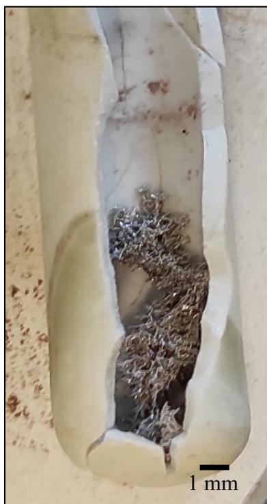
Fig.2: Broken  $\text{Ag}/\text{Ag}_2\text{SO}_4$  reference electrode after 195 h immersion in  $\text{Na}_2\text{SO}_4$  at  $900^\circ\text{C}$ . The photo displays the Ag sponge formed in place of the initially 1 mm in diameter Ag wire.
