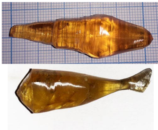
Figure 2. Photographs of the as-grown crystal boules of (a) undoped \text{MgMoO}_4 and (b) 0.1 at.% \text{Tm}^{3+} -doped \text{MgMoO}_4 (actual doping level). The growth direction is along the [001] axis.
