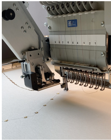
Fig. 2. Development of embroidery circuit with mounted LEDs.
