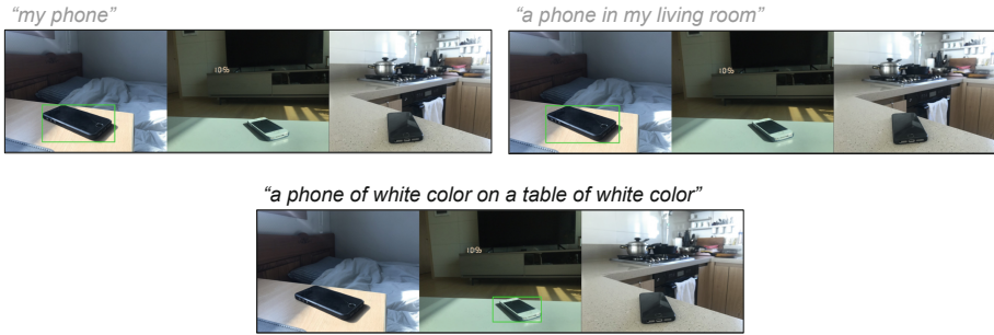
Fig. 2. Demo results of the up-to-date vision and language model dealing with referring expression comprehension [10]. Given images where the image in the middle is the user’s phone, the model failed to comprehend expressions that describe a personal relationship with the use of possessive words such as “my phone” or “a phone in my living room” (first row). However, the model could successfully detect the user’s phone when the expression was “a phone of white color on a table of white color” (second row).
