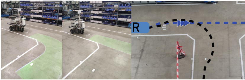
Fig. 2. Explicit (A, left) and implicit (B, right) communication tools compared in this study. Shown exemplary for the intersection scenario. The two dotted lines (for B) are the two trial variants.
