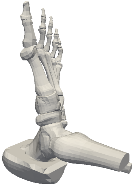
Figure 5: A part of a heel tissue model used in simulations in which its orientation corresponds to the situation when the patient is in bed.
