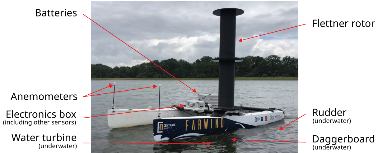
Fig. 3. The Farwind prototype with its instrumentation. The rudder, daggerboard and water turbine are not visible through the water surface.
