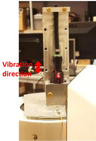
**Figure 3: Fixture and vibration direction (front view)**
