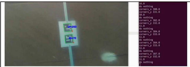
Fig. 7. ArUco codes detection by the camera of the BlueROV
