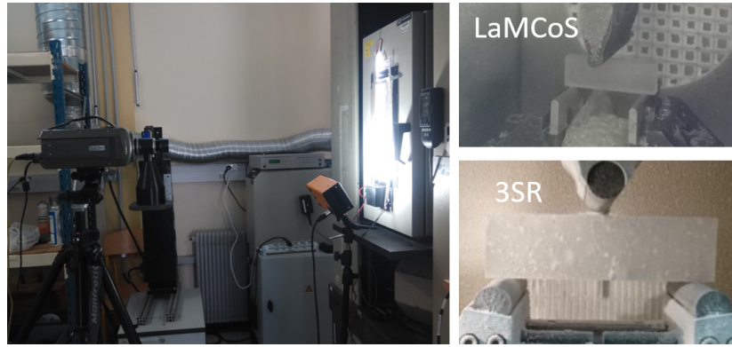
Figure 7: Left: High speed camera pointing toward the climatic enclosure (LaMCoS). Right: Three-points bending devices.
