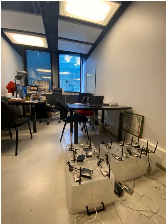
Fig. 5. Testing location and composition of the super-sniffer. The order in which we place our co-located sniffers to form a super-sniffer of maximum size 14.
