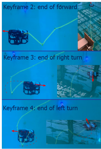
Fig. 11. Views of the overall system at different points along the curvilinear trajectory when the cable is controlled. The red arrows indicate the direction of motion of the ROV. (Video at https://youtu.be/fy-JTc8PvIY )
