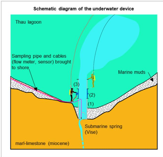
**Fig. 3.** Principle diagram (not to scale) of the instrumentation of the submarine spring in its context of emergence according to the diving explorations. (1): flow collector, (2): flowmeter, (3): stilling tube.
