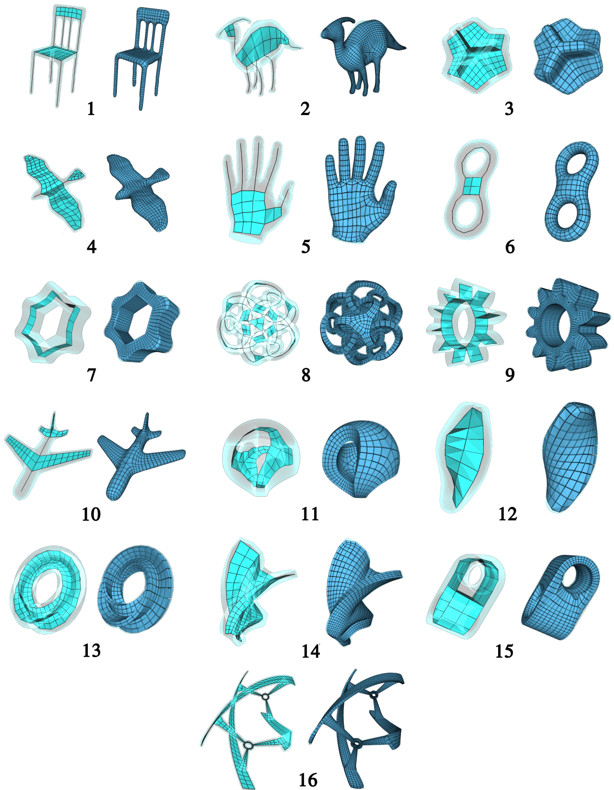
Figure 18: Several meshes obtained using our algorithm with post processing using padding, simple subdivision, and geometric optimization. For each model, the left image shows the silhouette of the domain and the meso-skeleton and the right image shows the obtained hex mesh. Quality measures for these meshes are indicated in Table 1.
