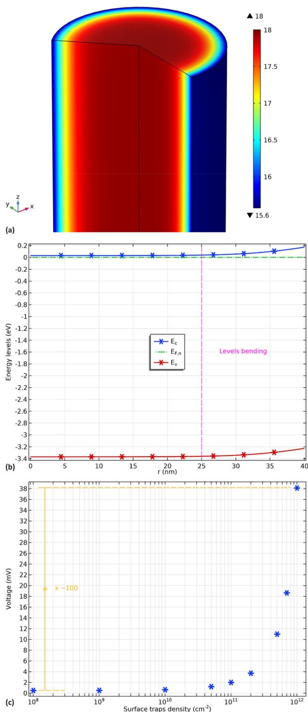
**Figure 6.** a) Electronic concentration and visualization of the depletion zone, b) Energy levels (in eV) in the function of the radial position, and c) Evolution of the open-circuit voltage between both ends of the NW in the function of the surface traps density (n-doping value  $10^{18} \text{ cm}^{-3}$ ).
