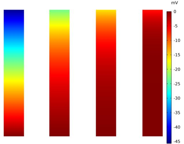
**Figure 4.** Comparison of piezo-potential distributions in a NW median plane in function of doping level (from left to right:  $10^{14}$ ,  $5 \times 10^{14}$ ,  $10^{15}$ , and  $5 \times 10^{15} \text{ cm}^{-3}$ ).
