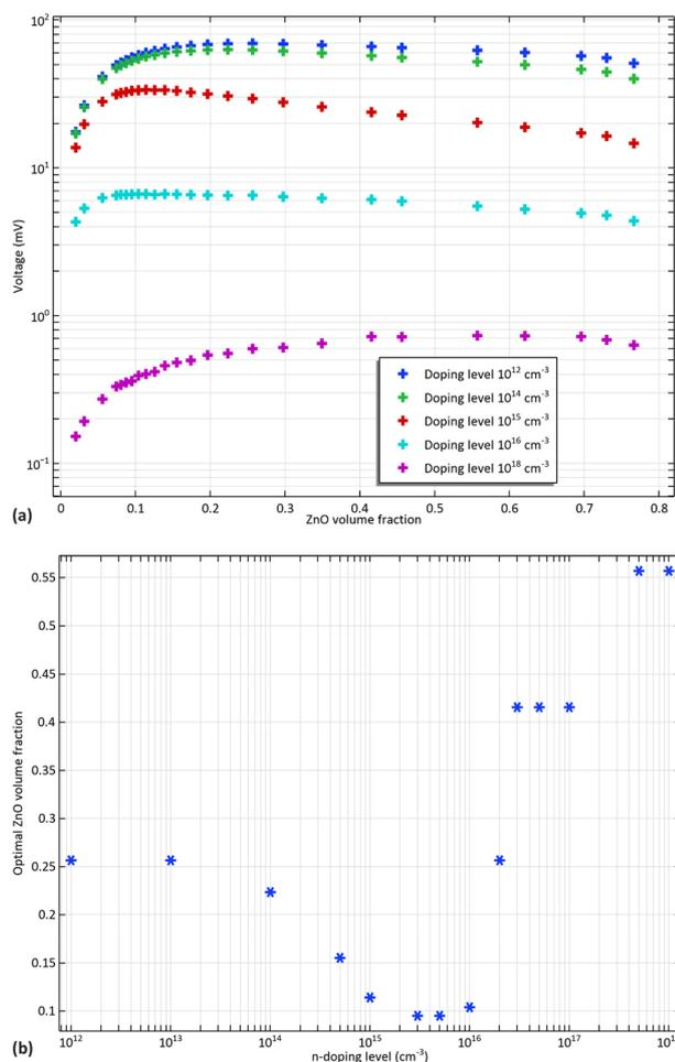
**Figure 11.** a) Evolution of the open-circuit voltage between both ends of the NW in the function of the ZnO fraction for different n-doping levels without surface traps b) Optimum ZnO volume fraction for different n-doping levels without surface traps.
