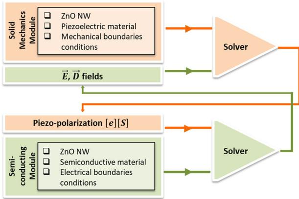
Figure 1. Principle diagram of the PZ-SC coupled model.
