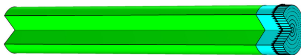
Figure 7. Schematic of the simulated structure (green: ZnO NW and cyan: polymer layer) with the compression load (black arrows).
