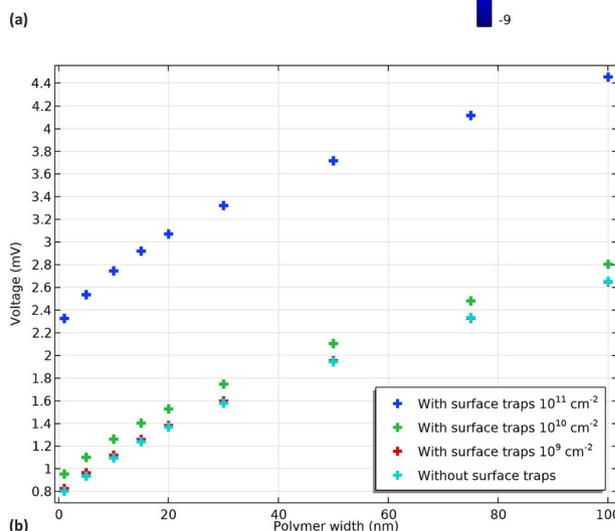
**Figure 9.** a) Piezopotential for a 75 nm polymer width and a  $10^{11} \text{ cm}^{-2}$  NW surface traps density (black arrows showing compression), b) Open-circuit voltage between both ends of the NW versus the polymer width for different surface traps density values.
