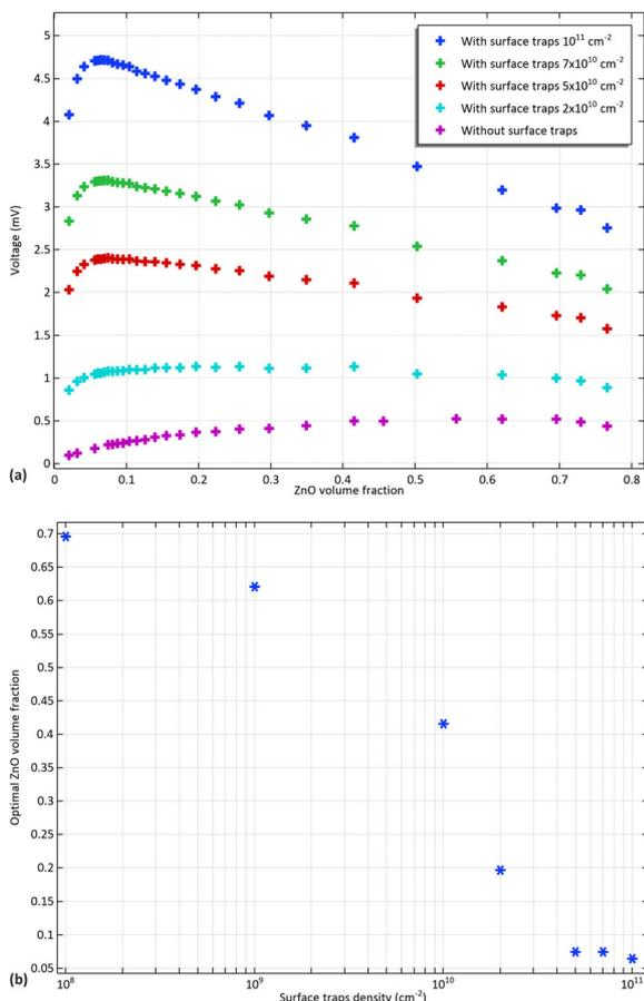
**Figure 13.** a) Evolution of the open-circuit voltage in function of the ZnO fraction for different surface traps densities and a n-doping level of  $10^{18} \text{ cm}^{-3}$  b) Optimum ZnO volume fraction for different surface traps densities and a n-doping level of  $10^{18} \text{ cm}^{-3}$ .
