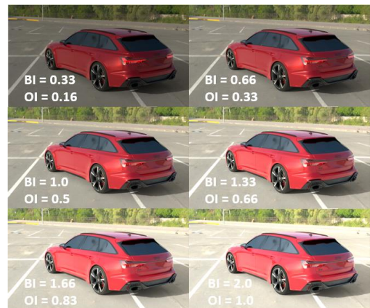
Figure 5. Different background intensities (BI) with adapted object intensity (OI)
