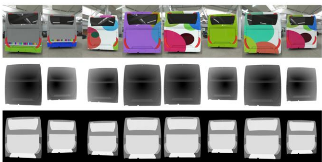
Figure 22. Dataset containing few bus back-ends RGB-D images generated with BlendGen using the ray tracing render engine named Cycles
