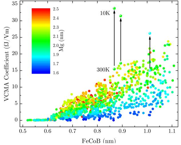
Fig. 6. Experimental variation of the VCMA coefficient  $\xi$  with effective FeCoB thickness of the storage layer and MgO tunnel barrier. The arrow represents the increase in VCMA measured on a single device at 5K.
