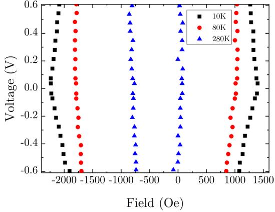
Fig. 5. Switching field boundaries for 280K, 80K and 10K in red, black and blue, respectively. The heating capacity reduction of MgO at low temperature is visible at 10K from the symmetrical effect  $V_b$  has on coercivity.
