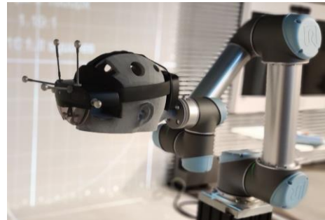
Figure 1: Picture of the 3D printed head installed on the UR5 with a Hololens 2 mounted on it.
