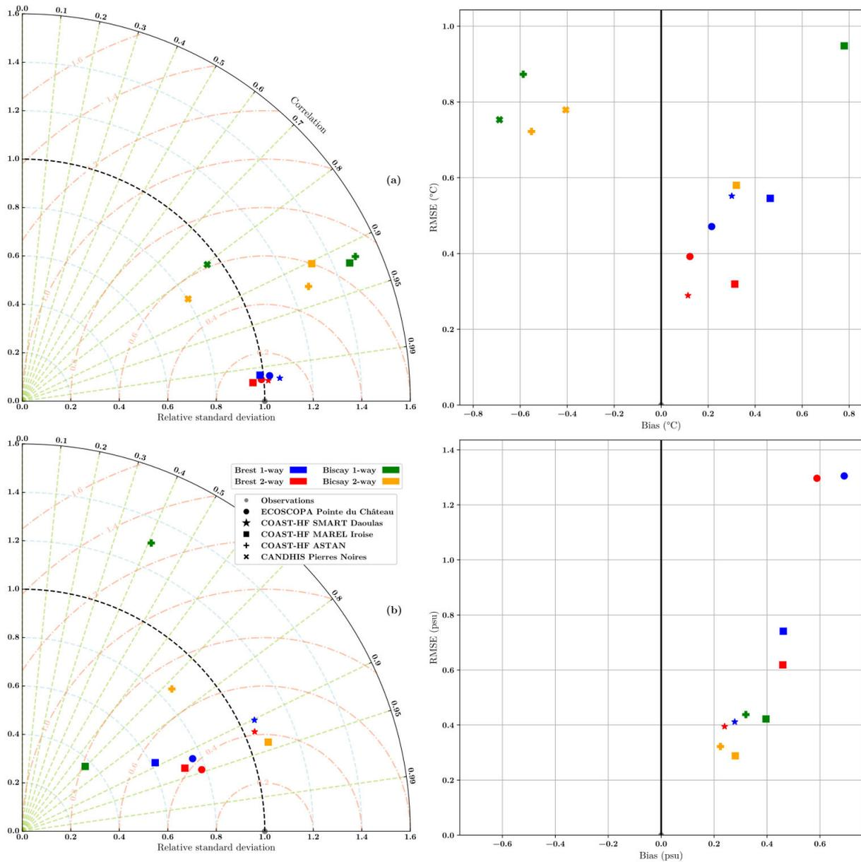
**Figure 6.** Temperature (a) and salinity (b) validation for both configurations. The Taylor diagrams are represented with the relative standard deviation (dashed blue lines), correlation (dashed green lines) and relative root mean square error (dashed red lines).
