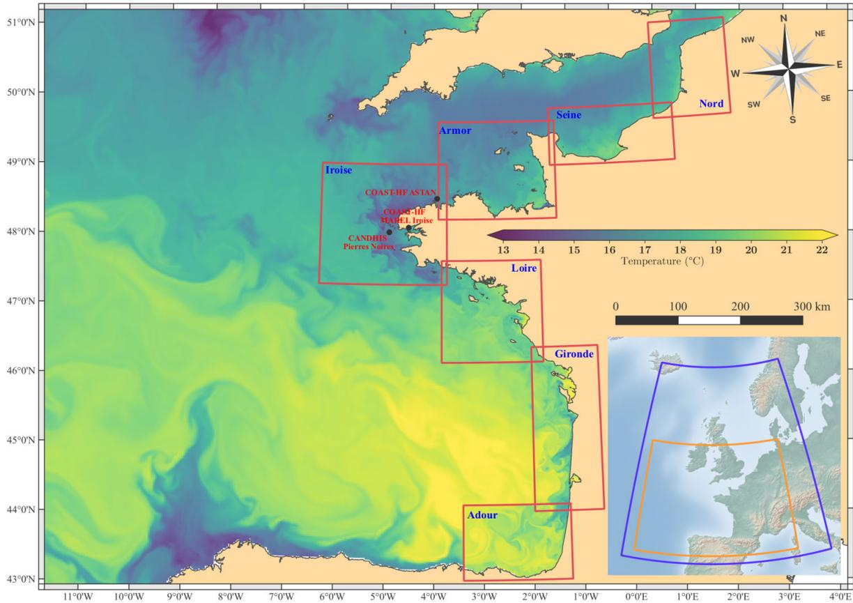
**Figure 5.** A Bay of Biscay configuration with seven magnified views at 500 m resolution (red rectangles). The 2.5 km resolution coarser grid (orange rectangle) is included in a larger 2D model at 5 km resolution (blue rectangle). The sea surface temperature is given for 16 August 2018 with the finest possible resolution. Bathymetric and coastline sources: Ifremer, Service hydrographique et océanographique de la marine (SHOM) and Natural Earth.
