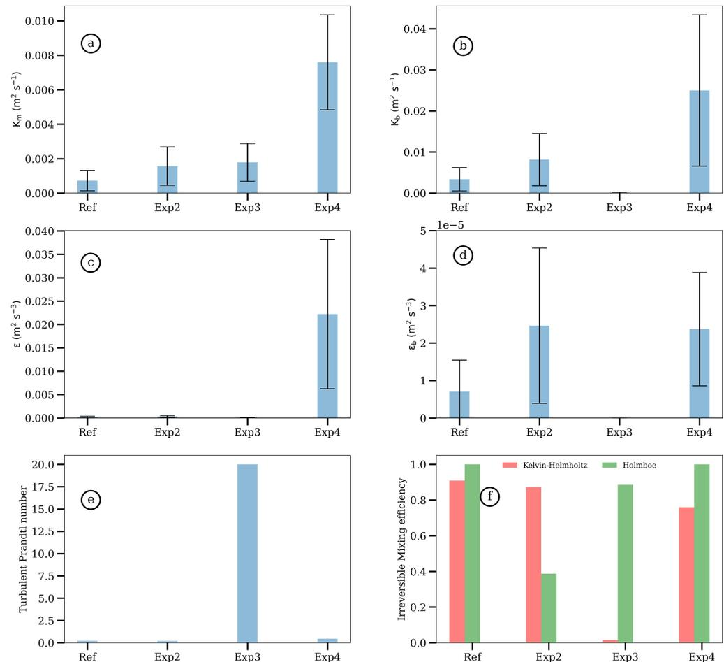
**Figure 13.** Statistics and error bars (vertical segments at the end of the colored lines) for all experiments: (a) vertical eddy viscosity, (b) vertical diffusivity, (c) vertical EKE dissipation, (d) vertical buoyancy dissipation, (e) turbulent Prandtl number, and (f) irreversible mixing efficiency for KH (red) and Holmboe (green) instabilities.
