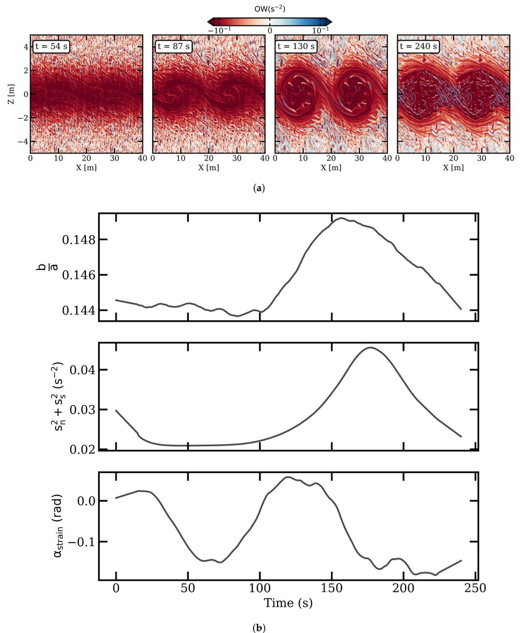
**Figure 3.** (a) Snapshots of the Okubo–Weiss parameter in the reference experiment. (b) Time evolution (reference experiment) of the aspect ratio of the two billows (**top row**), the intensity of the strain (**second row**), and its direction (**bottom row**).
