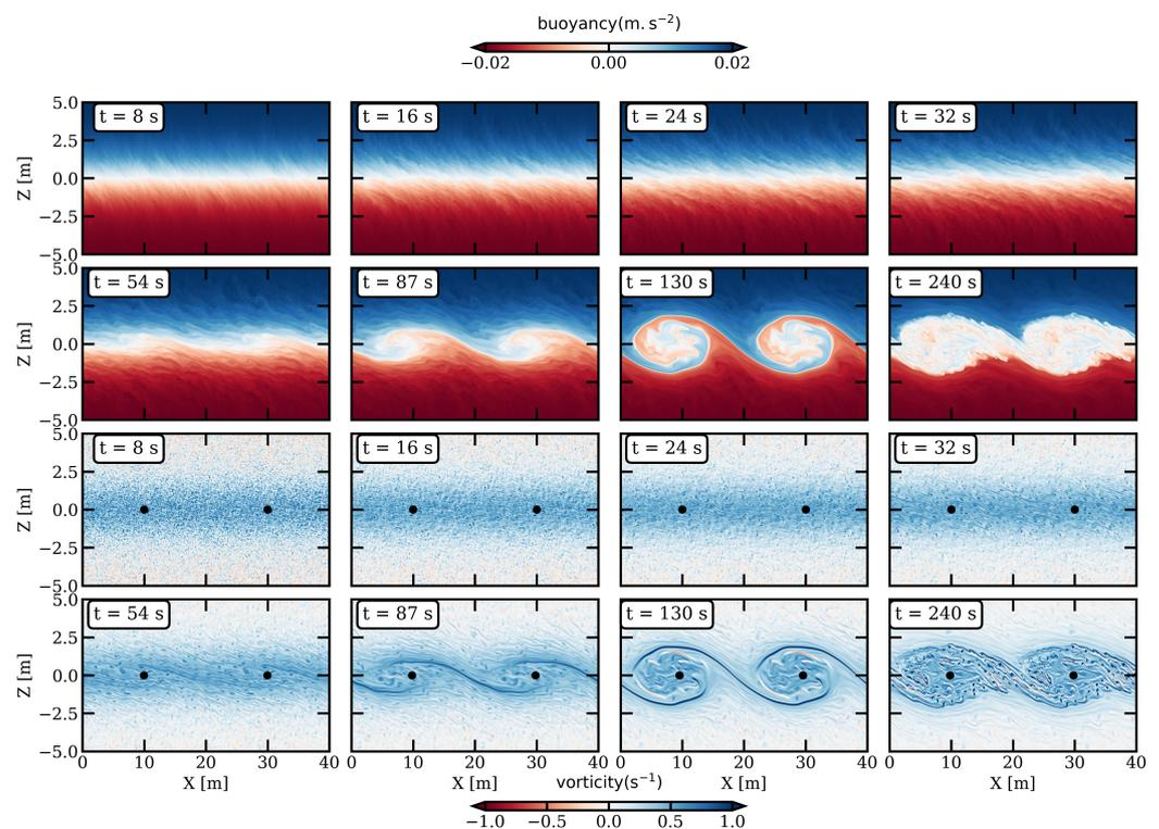
**Figure 2.** Snapshots from the reference experiment of: buoyancy field (**top two rows**), vorticity field (**bottom two rows**). The black dots in the vorticity field indicate the vorticity centroid of each billow.
