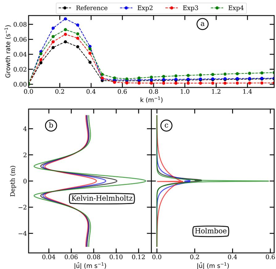
**Figure 10.** (a) The growth rate, (b) the vertical magnitude of the streamwise velocity for the Kelvin–Helmholtz mode, and (c) the vertical magnitude of the streamwise velocity for the Holmboe mode for the reference and sensitivity experiments.
