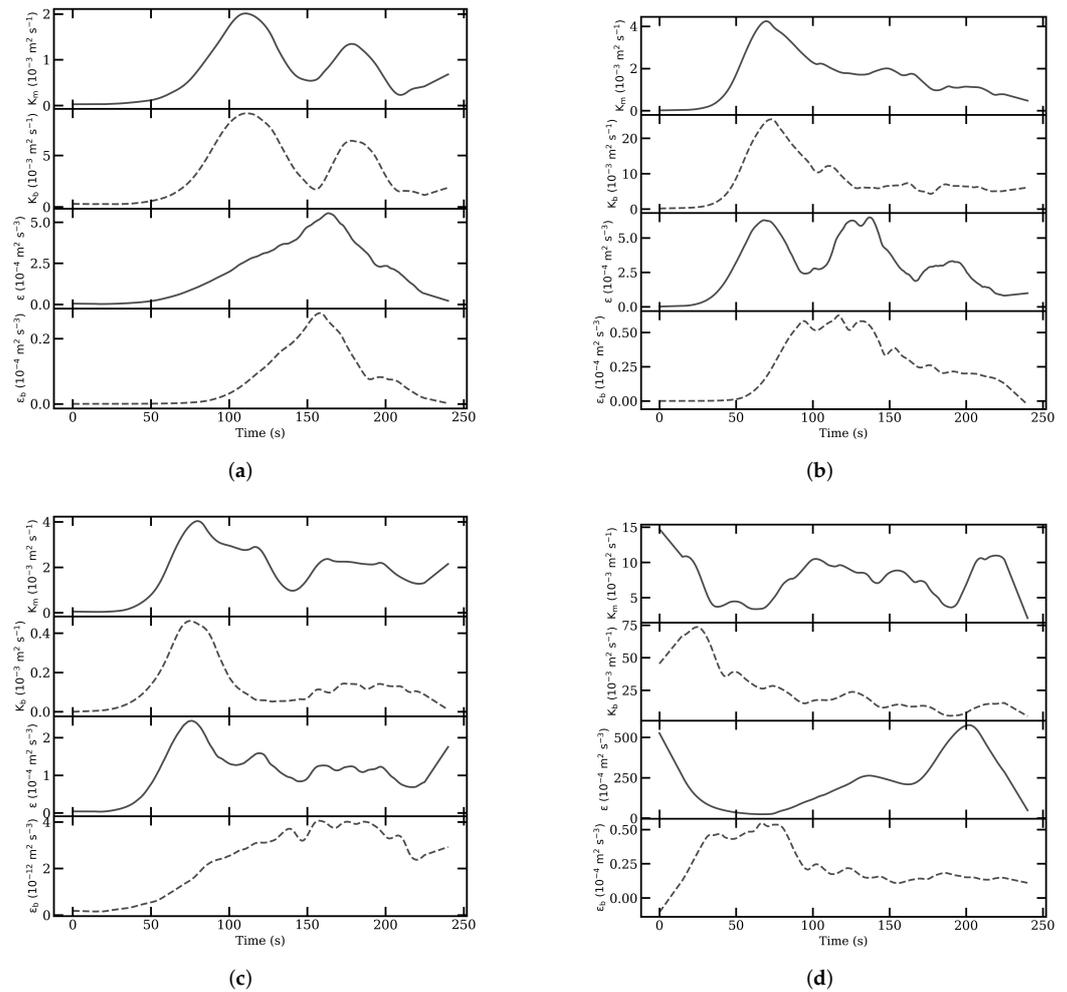
**Figure 12.** Vertical eddy viscosity (black solid line), vertical diffusivity (black dashed line), and vertical dissipation of EKE (black solid line) and buoyancy (black dashed line) for the reference configuration (a), experiment 2 (b), experiment 3 (c), and experiment 4 (d).
