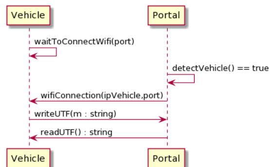
Figure 6: Interaction Portail/Véhicule
