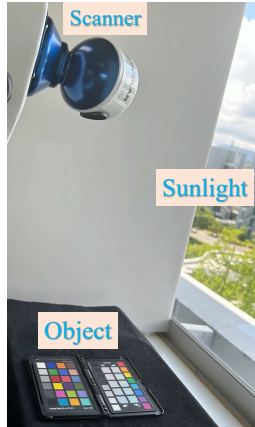
Figure 3: Experimental setup: The object is a colour chart of ColorCheckerPassport (X-rite, Inc) under uncontrollable illumination near a window.
