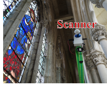
Figure 5: Experimental setup: Stained-glass window capture in Cathédrale Notre-Dame d'Amiens.
