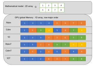
Fig. 2: Memory accesses according to the bloc configurations
